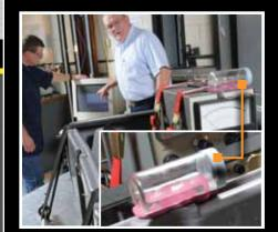
The water in the jar demonstrate to engineers the intense vibration a case withstands, while the jar attached to the equipment is calm, indicating a safe shock level (Shock mount technology does not apply to ProRack Cases).
